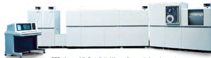
FCR, the world's first digital X-ray diagnostic imaging system
