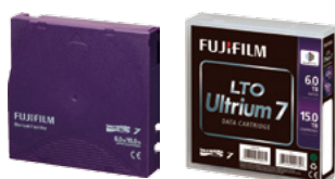
LTO Ultrium 7 data cartridge computer tape with BaFe magnetic particles
